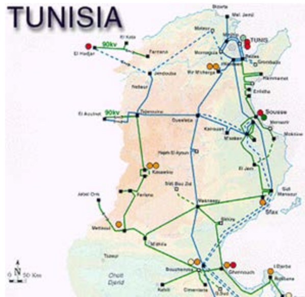
Figure 5 Tunisia's electricity network (GENI, 2013)
